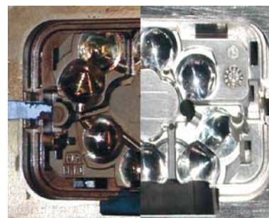
Ultrasonic cleaning of polished molding inserts
